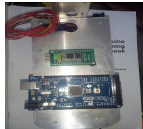
Figure 9: Assembly arduino Mega on robot & shield
